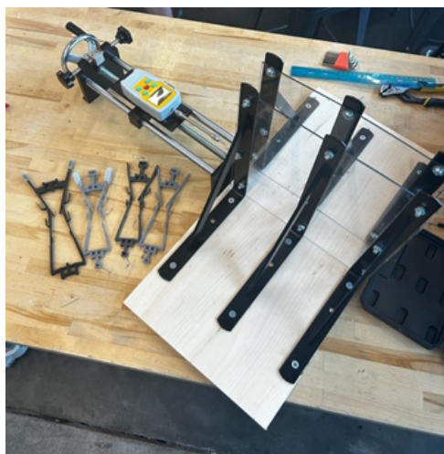
Figure 7: Test bed setup and hand-crank, pictured with printed legs. movement more challenging.
