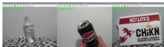
Figure 4: Raspberry Pi-5 camera live-time inference results.
